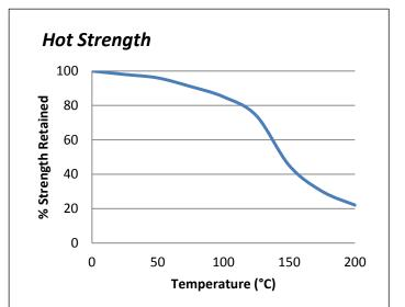
"Hot strength" shear strength tests performed on mild steel. Fully cured then conditioned to pull temperature for 30 minutes before testing. ES5741 can withstand higher temperatures for brief periods (such as for paint baking and wave soldering processes) providing the joint is not unduly stressed. The minimum temperature the cured adhesive can be exposed to is -40°C (-40°F) depending on the materials being bonded.
