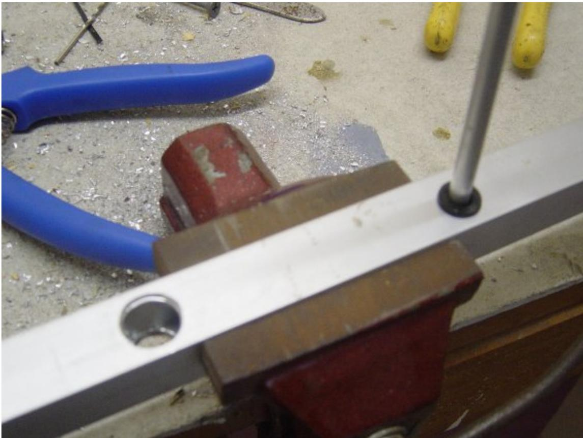
The boom was drilled using a drill press for accurate lining up, elements cut to size, and LED inserts trimmed. It was time to put it all together.
