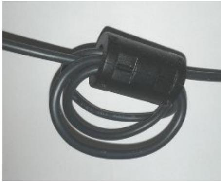
Clip it on your power cord as close to the ballast as you can get it, and loop the cord through a couple times. The impedance here rises as the square of the turns, so four (4) wraps are sixteen (16) times better than one wrap.
