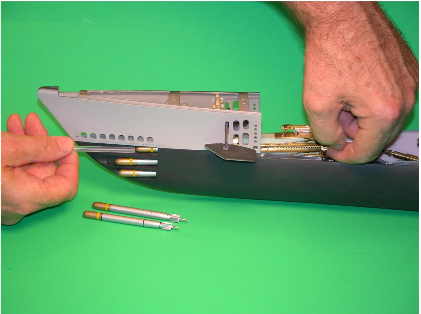
**Charging the Weapon** The system is so designed that you can not charge the weapon off-launcher. If the launcher is wet from recent immersion, insure that you blow out the little bit of water trapped within the face of the launcher charge fitting – failure to do so will result in water being driven into the system plumbing during the charging operation. If any water gets within the weapon it may flash to ice crystals as the propellant
