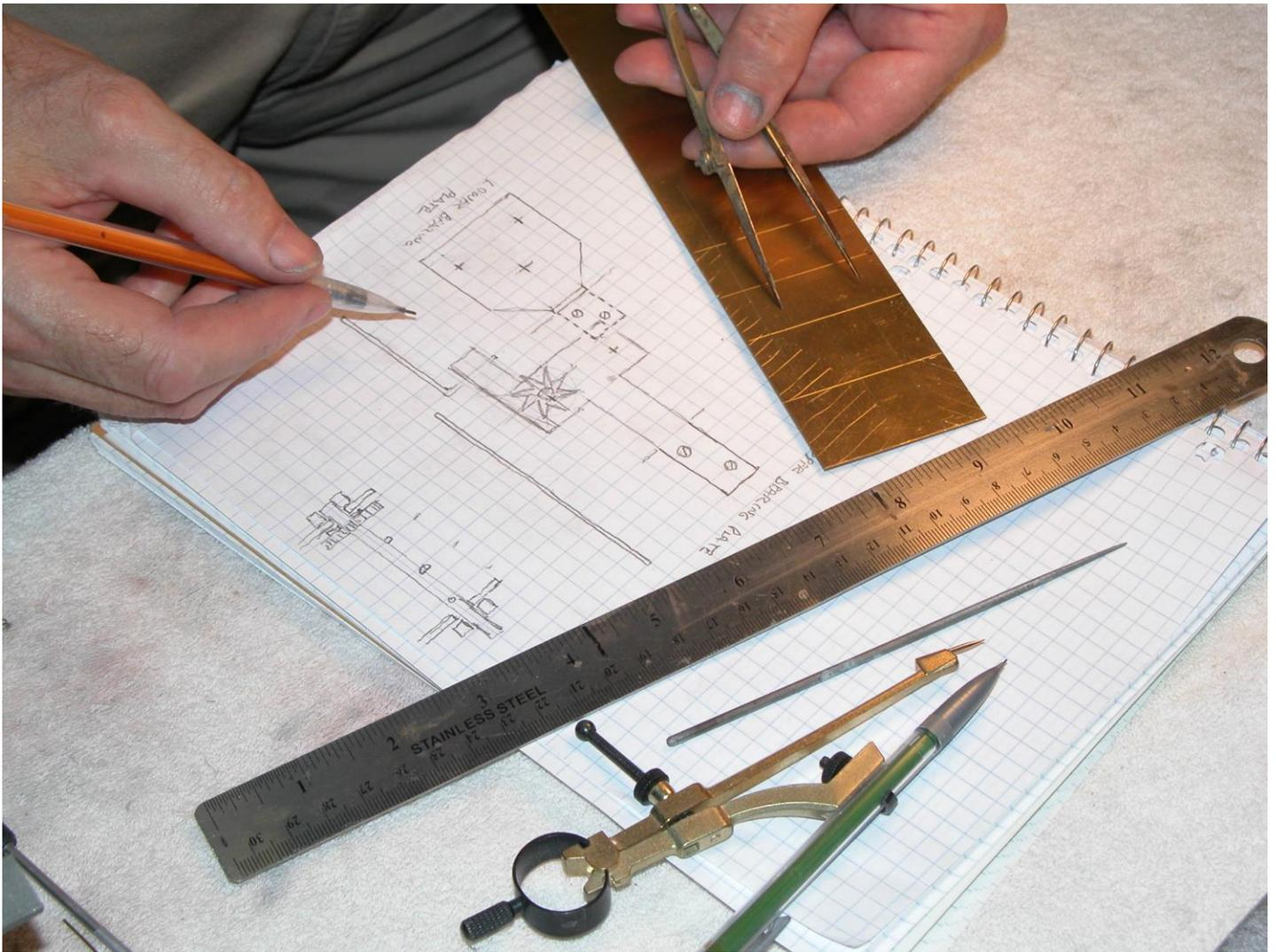
The geometry of the parts driven by function by the need to make clearance for the per-existing linkages, hull structure, and fittings within the bow of the GATO model. As it turned out the rearward face of the launcher nest foundation was the perfect mounting point for the launcher trigger tripping mechanism – the entire launcher trigger tripping mechanism could be removed quickly by pulling only four little machine screws that secured the two bearing plates to the launcher nest foundation.
