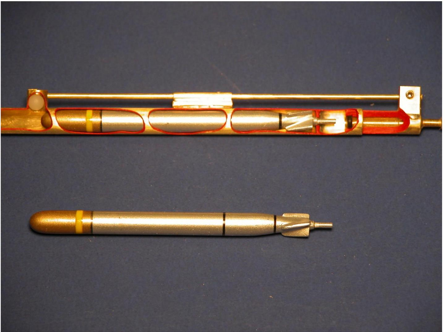
The launcher is designed for easy disassembly should the need arise for adjustment or repair. We have provided spare O-rings, stop-bolt ball, and an extra wheel-collar set-screw. Note in the picture below an assembled launcher in the battery condition. A disassembled launcher is presented above the assembled launcher. This shot should pretty much tell you all you need to know about launcher design and operation.
