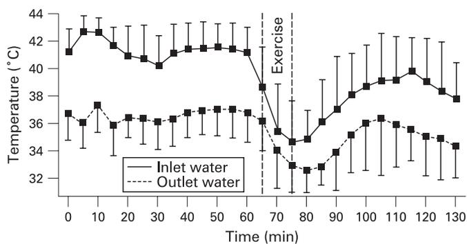
**Figure 1** Mean (SD) inlet and outlet temperature of the liquid conditioning garment over time. Values represent 5 minute means derived from data collected every 8 seconds.
