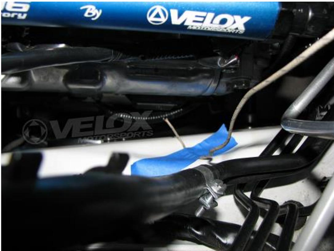
Fig. 5: Driver side coil thermocouple taped in place.
