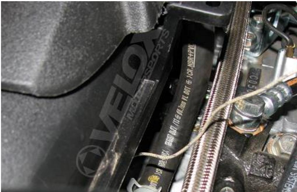
Fig. 7: Intake manifold thermocouple placement.
