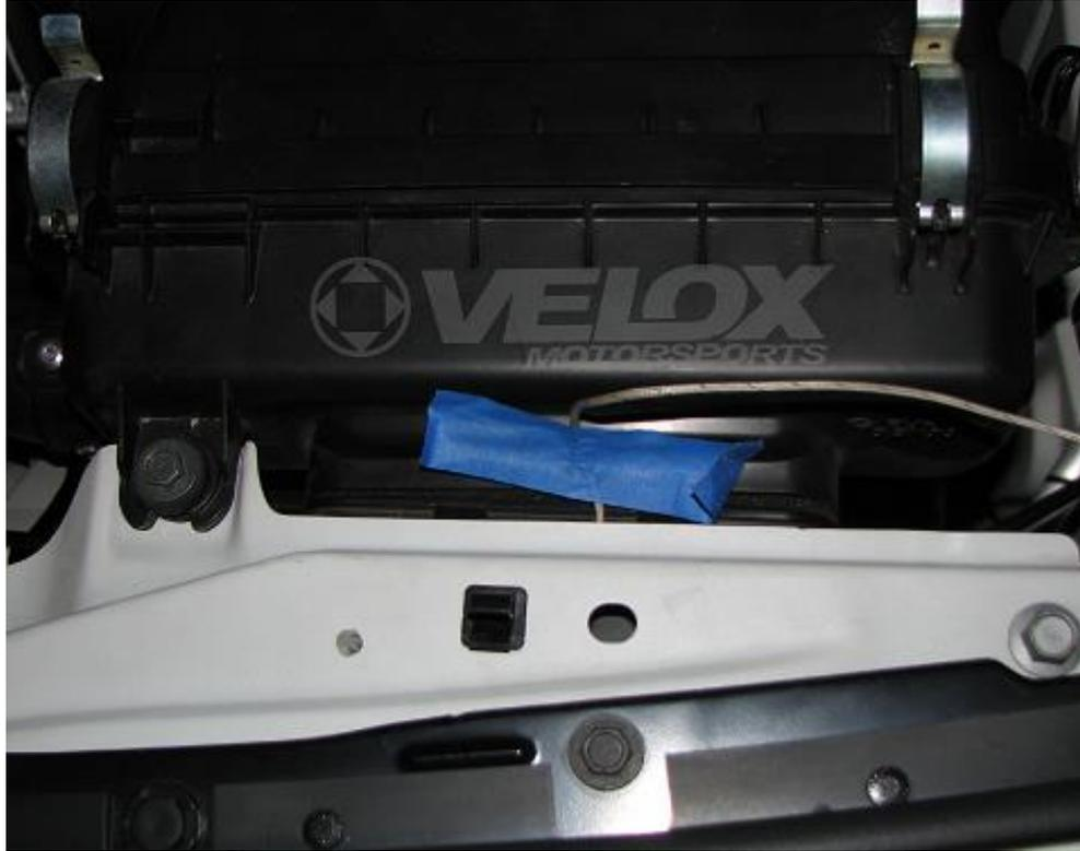
Fig. 6: Air box thermocouple taped into place.
