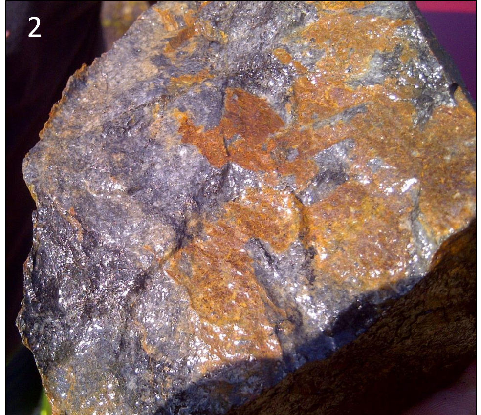
Hand sample of gold mineralized boulder. Disseminated pyrrhotite and arsenopyrite hosted in altered felsic volcanics. Assays up to 8.52 g/t Au
