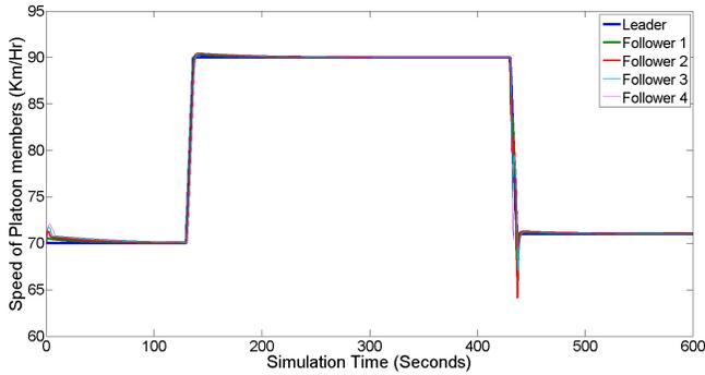
Fig. 3: Five vehicle Platoon velocity tracking
