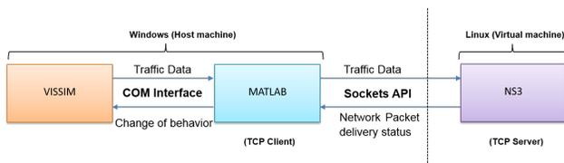
Fig. 1: Block diagram of the simulation environment.
