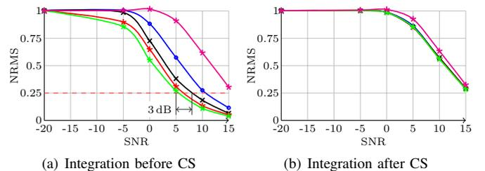
Fig. 1. Reconstruction error performance for integration (a) before, and (b) after CS reconstruction for the different coherent integration durations,  $N = 1$  (magenta),  $N = 5$  (blue),  $N = 10$  (black),  $N = 15$  (red), and  $N = 20$  (green). NRMS stands for normalized root-mean-square between the original and reconstructed target scene.
