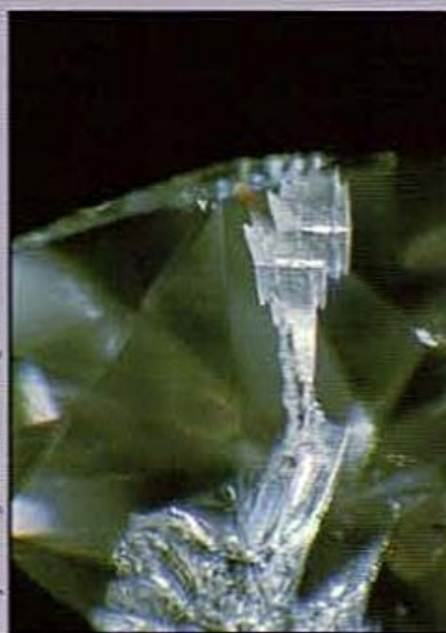
Figure 3: It is possible to see here how the laser-drill "trough" tapers as it goes from the surface of the stone to the inclusion.
