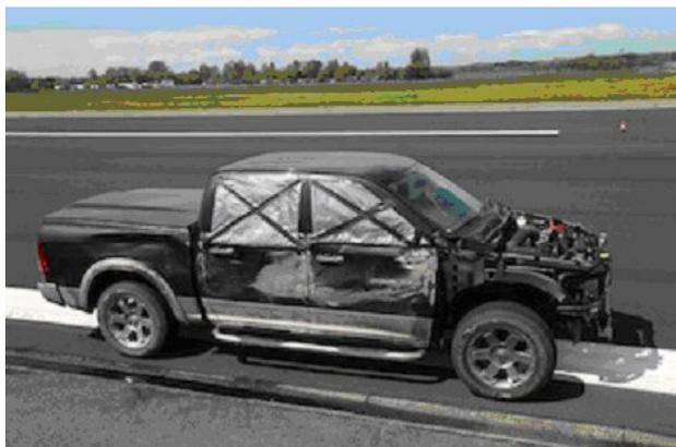
FIGURE 1: Dodge Ram 1500 accident vehicle used for validation testing
