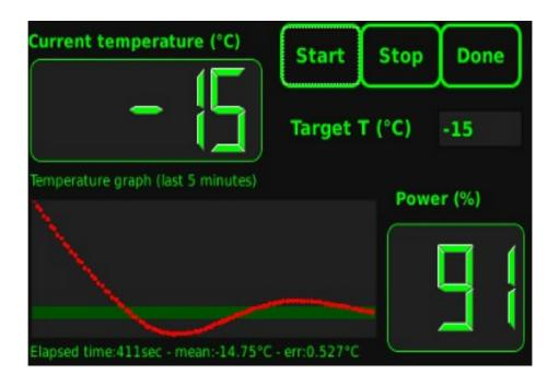
Push Done to leave the application: leaving the application doesn't stop the cooling process. Next time you open the Temperature Monitor application it will display the current cooling process state, until you push the Stop button, which will ramp down and
