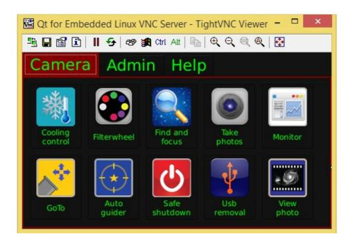
The camera automatically senses the presence of the touch LCD monitor at boot. When the monitor is not detected, the applications are started in VNC server mode and can be accessed by a VNC client.
