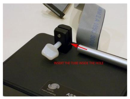
You can lock the monitor in the right position using the 2 white plastic knobs. Always be sure to lock the monitor properly to avoid movement during the exposures.
