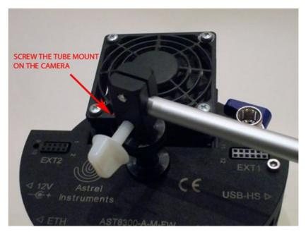
Mount the monitor as indicated in the pictures below: start by mounting the connecting tube to the back of the camera.
