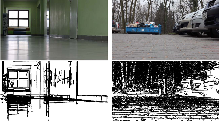
Fig. 1. Exemplary video frames for the indoor and outdoor sequences with results of Canny edge detection after dilation using 5 \times 5 pixels structuring element
