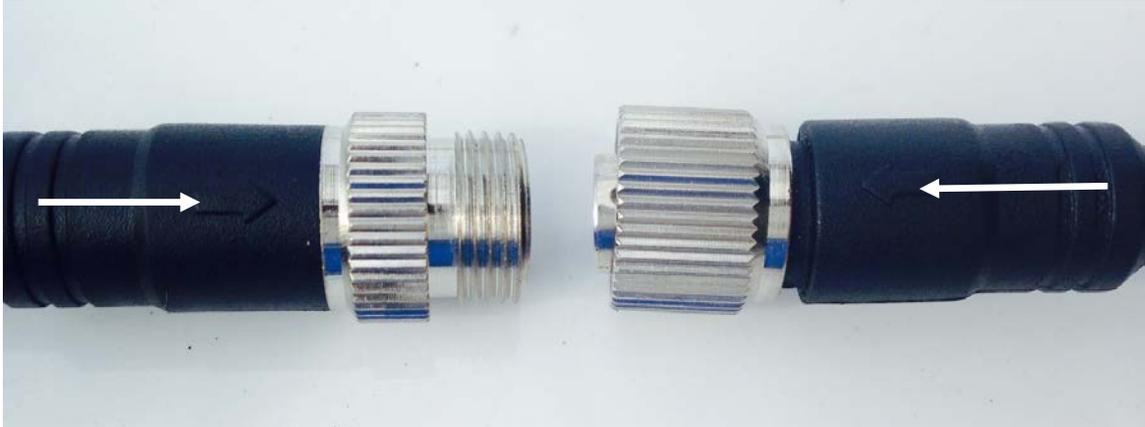
Turn silver cable connector nut clockwise to secure the connection of the cables. Do not over tighten. Ref. Fig.3 & Fig.2
