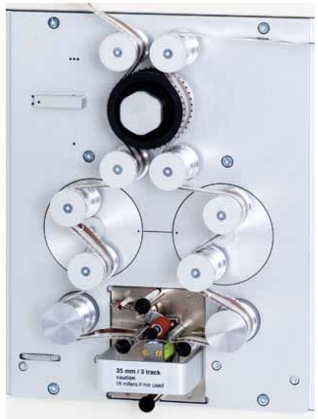
the closed-loop film drive ensures the efficiency of the archival additions to reproduce warped and shrunk stock in best possible quality
