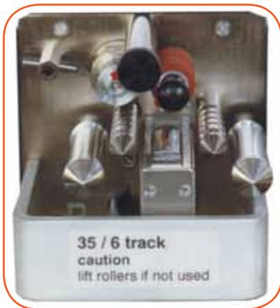
35mm headblock with retractable pressure roller and precision-machined rollers to straighten warped film and ensure proper film-to-head contact
