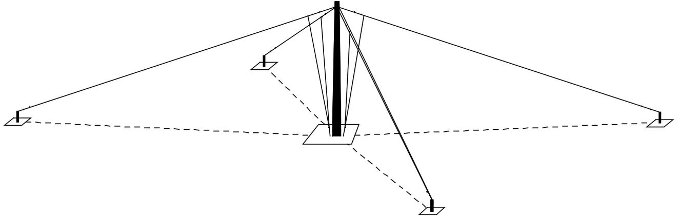
The Type OV2-30 is an omnidirectional wire antenna system that covers a base area of approximately 7200 sq m. (85 x 85) with a central mast approximately 20 metres tall. It has a continuous power supply capability of up to 1kW in the frequency range 2 to 30 MHz. It is designed to provide efficient and reliable communications in the professional/military services and is normally custom configured to suit site and communications parameters.
