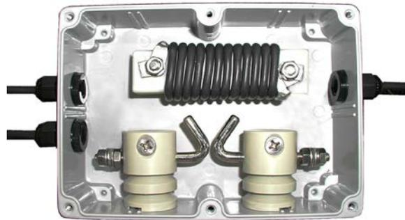
The Moonraker LPU is a horn gap overvoltage lightning protection system designed to be placed in MF/HF open wire antenna feeders. It gives an easy path to earth for high voltage static charges, such as those induced in the antenna system by lightning induction and other electromagnetic disturbances. When used with the CSS Coaxial Surge Suppressor, the range is extended to cover all frequencies from MF to 2 GHz.
