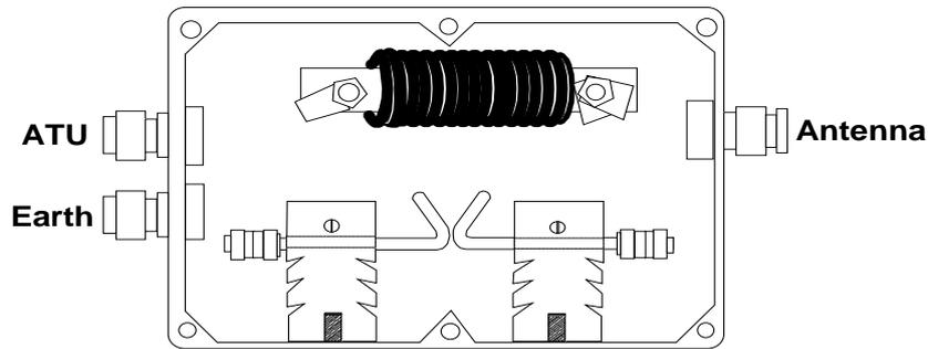
The unit is designed to be placed in the open wire feeder between the antenna and antenna tuning unit (ATU). A close by, low resistance earth point is essential for optimum protection.
