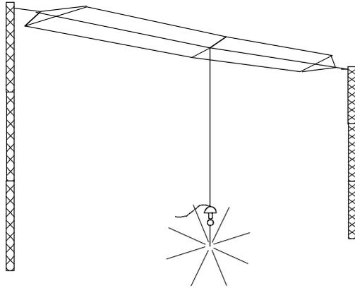
Designed as a higher efficiency alternative to vertical radiators, the T Top is a wire capacitive top antenna system for NDB and Differential GPS transmissions in the MF Band.
