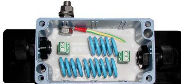
Lightning generated transients or overvoltages appearing across DC or AC cables and between them and earth are likely to be damaging to connected equipment. DC and AC external cables feeding navigation lights, wind speed and direction indicators, etc., can also carry these transient over voltages via the ships DC or AC wiring to other instruments and electronic devices such as chart plotters, computers, radios and the like, to cause damage.
