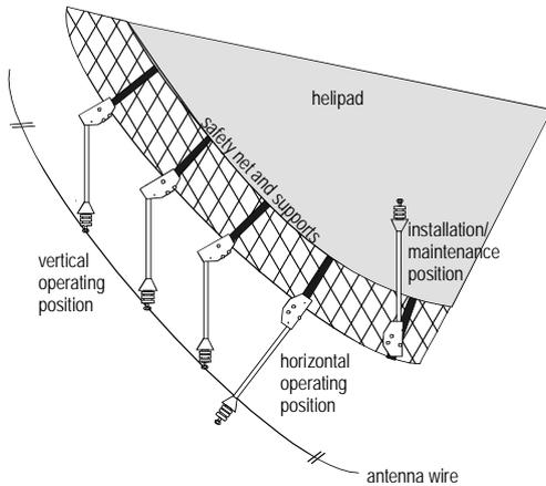
The HD MF antenna system extends around the perimeter of the helicopter landing pad at or below deck level. The system comprises multi strand hard drawn copper wire radiating element, which is supported by a number of tubular standoffs and insulators.
