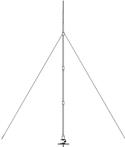
The 9.5M is practical to transport and easily erected and dismantled by the individual, being assembled from 2m (6.5ft) lengths. Roof mounting in city locations is both convenient and unobtrusive. Tempered corrosion resistant aluminium alloy tubing 32mm (1.25in) at base, tapering to 16mm (5/8in) at top, provides a large low loss radiating surface and, when trapped and/or loaded, extreme high efficiency is achieved. A low loss polypropylene insulator is fitted at the base.
