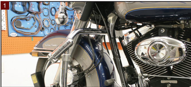
The Kiwi Tie-Down Anchors will be installed on the frame just forward of and below the gas tank.
