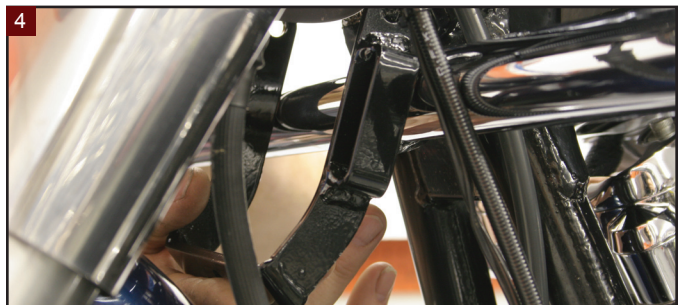
Carefully slide the Kiwi anchor behind the fork and over the engine guard.
