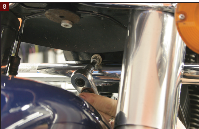
8 Thread the engine guard bolt into place and tighten it.
