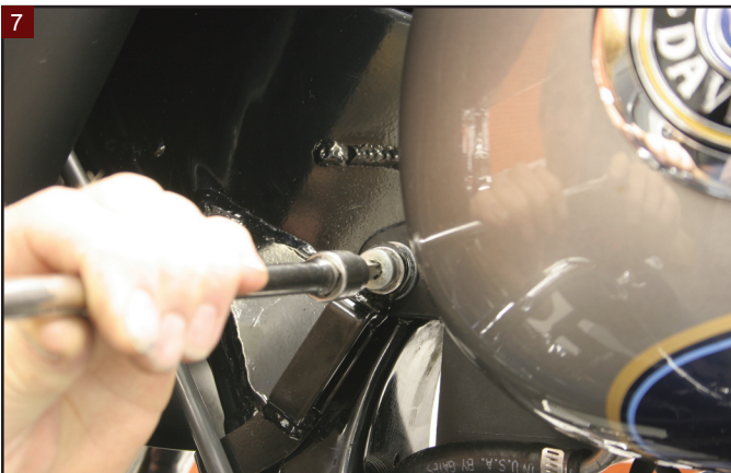
7 Place the large washers (included) between the tank mount tab and the frame. Thread the tank mount bolt into place and tighten it.
