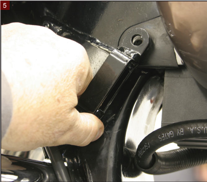
5 Align the holes in the bracket with the holes in the tank mounting tabs.
