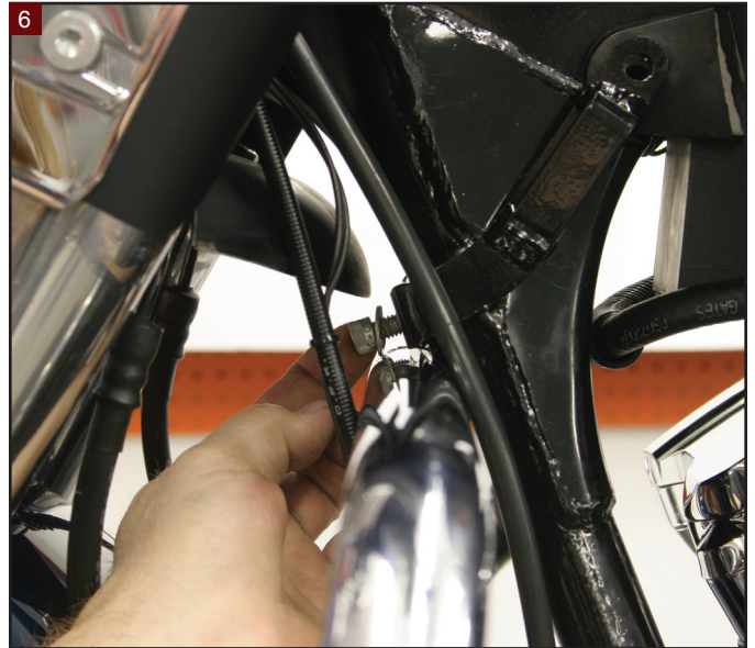
6 Thread the engine guard bolt into place to hold the Kiwi anchor in position.
