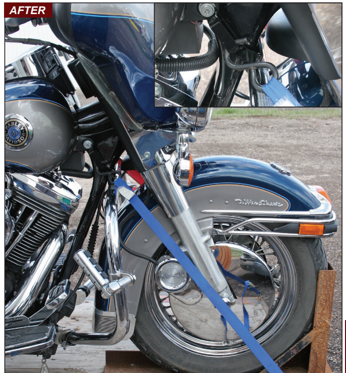
6 Thread the engine guard bolt into place to hold the Kiwi anchor in position.
