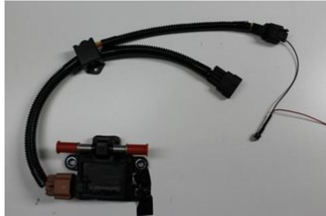
**The Smart Cable can be mounted in the vehicle's engine bay. While the unit is completely sealed, do keep away from any heat and water. The ideal mounting location for the analyzer box is in the battery compartment within reach of the vehicle grey 4 pole secondary air injection harness connector as pictured below, left.**
