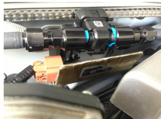
**If installing along with a vehicle flex fuel sensor, it is your responsibility to ensure that the fuel system components are installed correctly. Always check for fuel leaks. Seek professional installation if you are unsure, to avoid fire hazard. Ensure that the Smart Cable brown connector is within reach of the Ethanol Content Sensor.**
