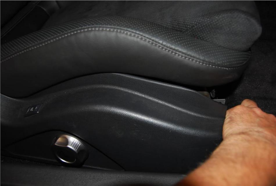
3. This is the 8mm hole already in the steel seat frame that is not being used for anything. It is at the tip of my index finger. This is where the end of the s bent bracket will be fastened.
