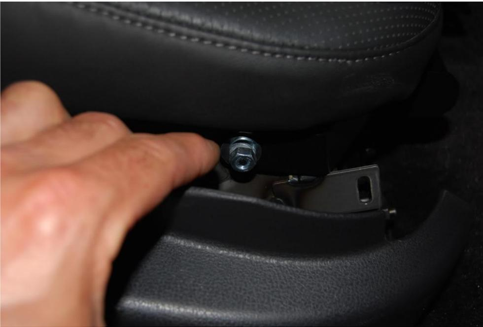
9. Tighten the L shaped bracket on the other end of the mount by tightening the hex bolt first, and then the nut and lock washer. Finish by snapping the trim back into place. It should look like this.....ready for an extinguisher.
