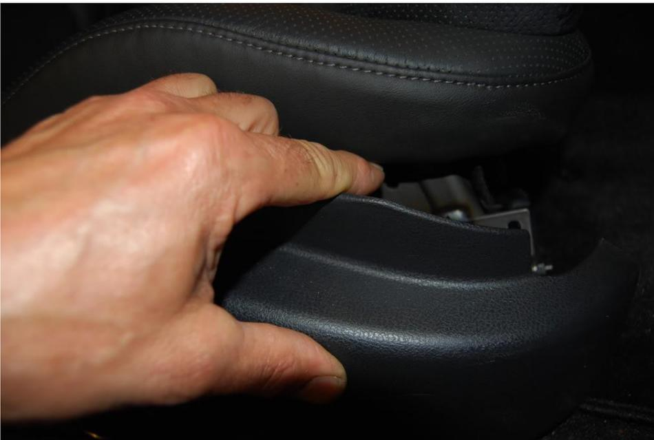
4. There is a triangular bracket that is not being used for anything that is under the left forward part of the seat. This is where the L shaped rounded bracket fastens. There is a 6mm hole towards the front of it. The tip of my finger is on it.
