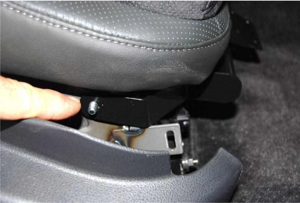
8. Place a washer on the hex bolt along with a split washer and nut. You can get a wrench on the backside and then tighten the s mount side. 7/16" ratchet wrench is really helpful doing this install, but not needed. You can tighten this now.
