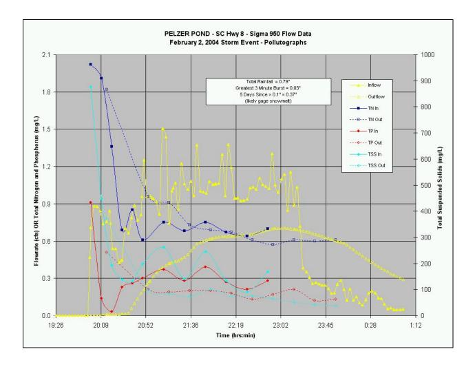
After downloading this data above from each flow meter after each measured storm event, numerous calculations were completed in Excel to determine the total flow volume at both the inlet and outlet.
