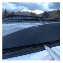
Use a knife, flathead screwdriver or other flat figid object to pry the covers off the stock roof rack. Place a rag or paper towel over the paint so you can pry against the vehicle without scratching the paint.
