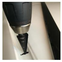
After marking the hole with a center punch, use a step drill bit to begin drilling (You will drill till the 3/8" level pierces the top of the roof). MEASURE TWICE, DRILL ONCE! You need to make sure you drill the hole far enough from the sides of the channel for the spacer to fit.
