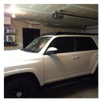
Make sure the rack is centered and loosely secured at all mounting points. Once the rack is in the desired location. Tighten each bolt till the lock washer is fully compressed and spacer is firmly seated against the roof.
