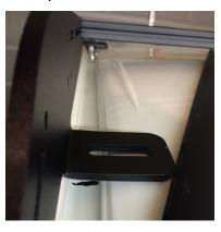
Using a marker. Mark the location of the slot using a horizontal line accross the roof channel where the front mounting point will be.
