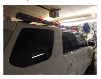
To mark the front mounting hole you will first need to semi assemble the rack. Do this by bolting in three crossbars as shown on page 3 in the locations shown above. Once this step is complete. Place the rack on the vehicle's roof resting it on the spacers.
