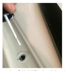
Once you have finished drilling through the roof to the 3/8" with the step bit, finish the hole with a standard 3/8" bit to make sure the hole is even all the way through. Use some touch up paint to cover the exposed metal as much as possible. Repeat this step on the other side of the vehicle.
