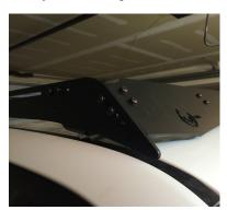
Weather strips in the front can be cut with tin snips to the correct length to fit around the spacers for the front mounting points.
