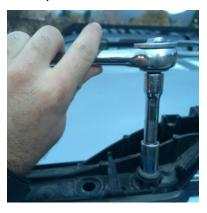
Remove the hex bolts holding the factory roof rack to the vehicle.
