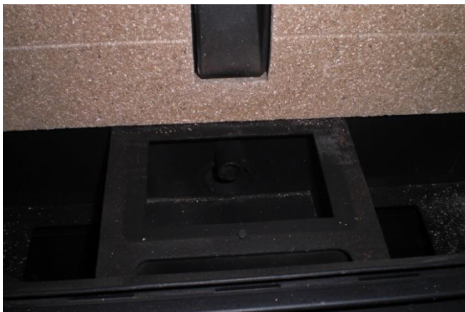
Figure 35: Remove ash from ignitor tube (underneath repot)
