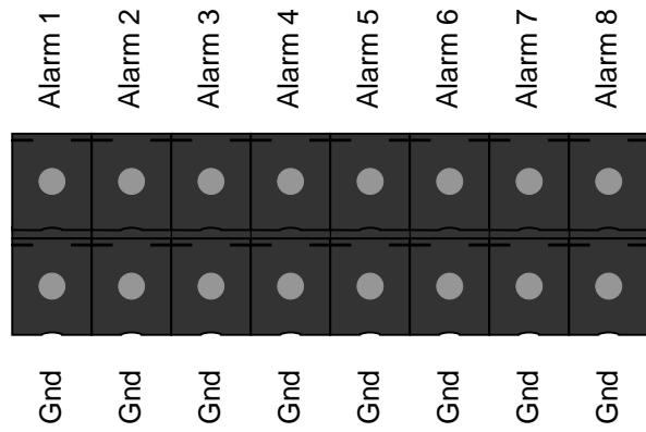
Above is the pin out of the connector on the rear of physical interface, you can see that each alarm input has its own corresponding ground. All the grounds are on a common bus and all alarm inputs can be taken back to a single ground connector if this makes installation easier.
