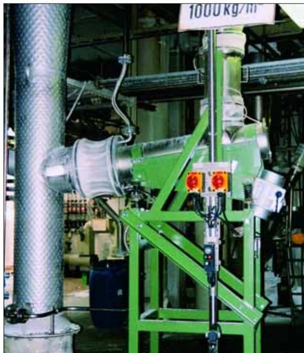
Fig. 16 Vibrating tube conveyor with water-cooled outlet and water-cooled downpipe
