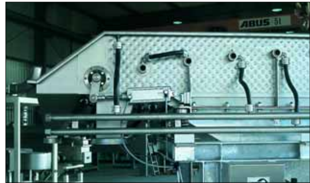
Fig. 17 Screen case with heated walls and screen supports to prevent caking
