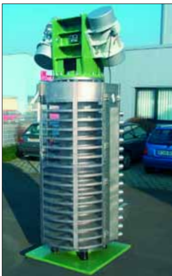
Fig. 21 Spiral conveyor with transparent dust cover and cooling air connections
