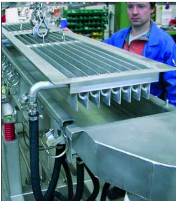
Figs. 3 and 4 Water-cooled vibrating trough conveyor with additional heat exchanger inserts
