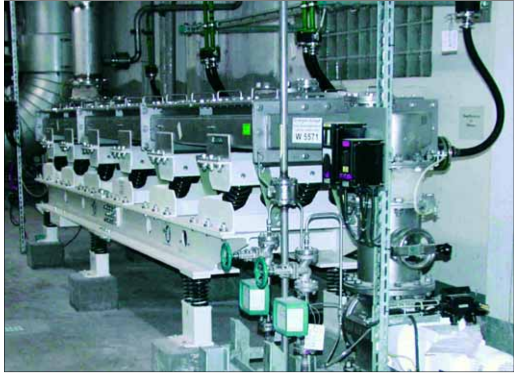
Fig. 14 The temperatures and temperature profiles of the decks can be electronically monitored and controlled
