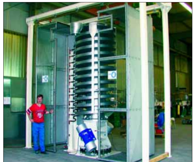
Fig. 23 Spiral conveyor with transparent dust cover / noise reducing enclosure. The enclosure consists of two moving halves suspended on rails which can be separated for cleaning
