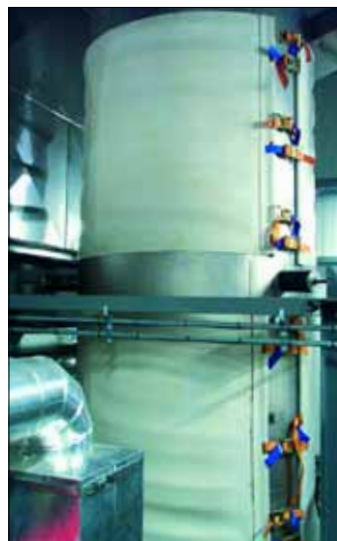
Fig. 22 Spiral conveyor with natural rubber dust cover
