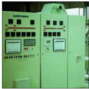
Fig. 14 The temperatures and temperature profiles of the decks can be electronically monitored and controlled
