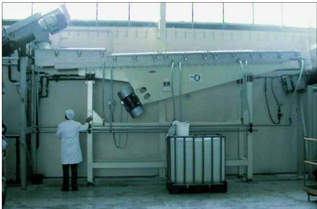
Fig. 9 Cooling trough conveyor for dusting powder – food grade design with integrated product buffer for batchwise feeding and continuous further processing
