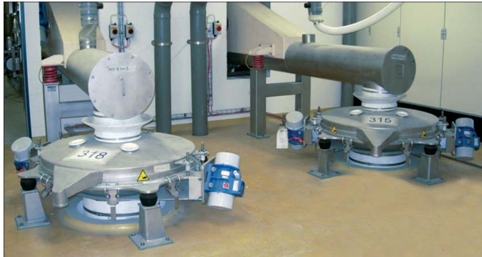
Round screening machines for screening salt
