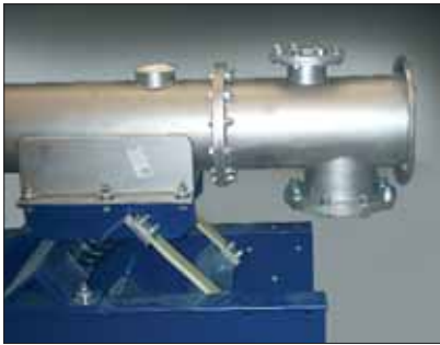
Fig. 19 The modular design allows the conveying line to be subsequently extended if required
