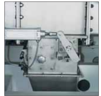
Fig. 25 Flap element flanged into the conveyor trough
