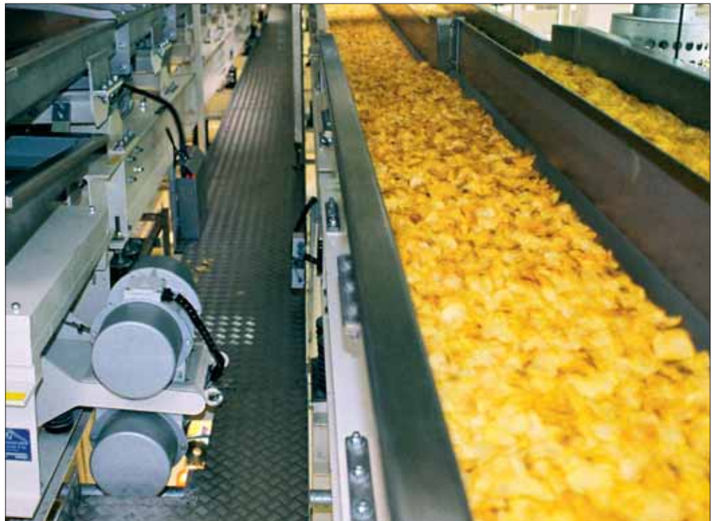
Fig. 28 Figures 27 and 28 are partial views of a machine with water-cooled natural frequency trough conveyors for cooling 15 t/h of roasted product down from 800°C
