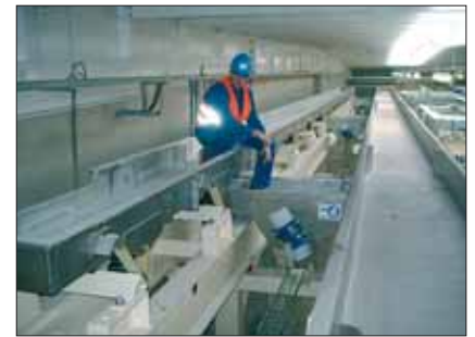
Fig. 18 Assembly line for a vibrating conveyor for cereals with an overall length of 80 m
