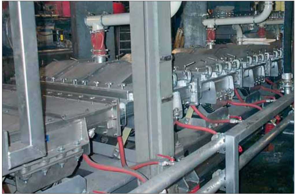
Fig. 28 Figures 27 and 28 are partial views of a machine with water-cooled natural frequency trough conveyors for cooling 15 t/h of roasted product down from 800°C
