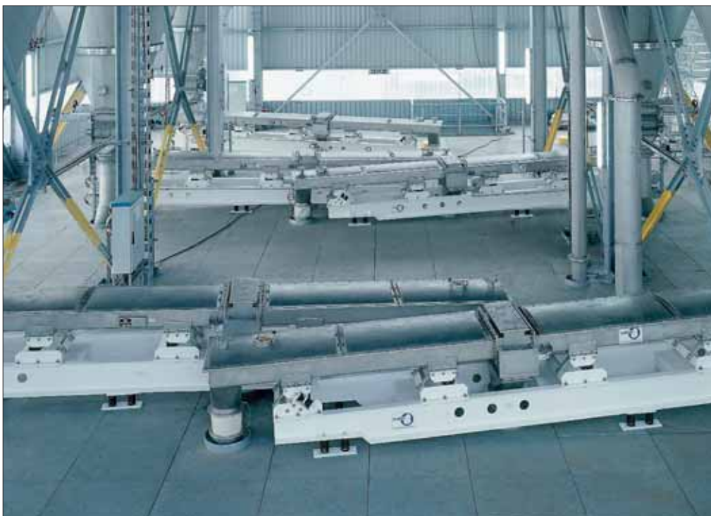
Fig. 9 Six natural frequency trough conveyors for transporting material between the silos and the loading station
