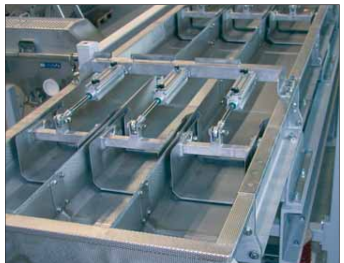
Fig. 26 Multiple-track trough conveyor with nine discharge flaps for feeding packaging machines
