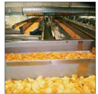
Fig. 10 Natural frequency trough conveyors for handling 50 m 3 /h of potato chips
