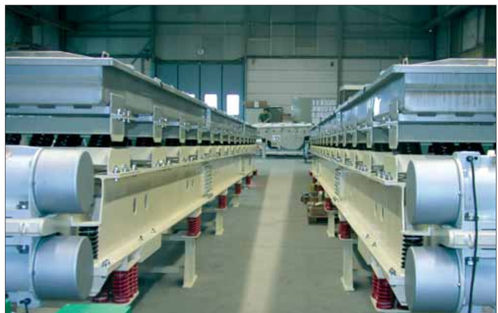
Fig. 31 20 m long natural fre- quency conveyors for handling 40 t/h of steamed rice
