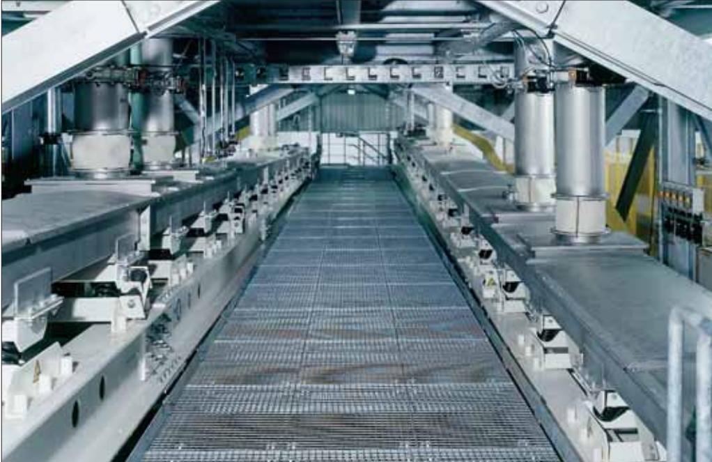
Fig. 4 Figures 4 and 6 show two natural frequency trough conveyors, 800 mm wide x 26 m long, for handling 50 m 3 /h of filler
