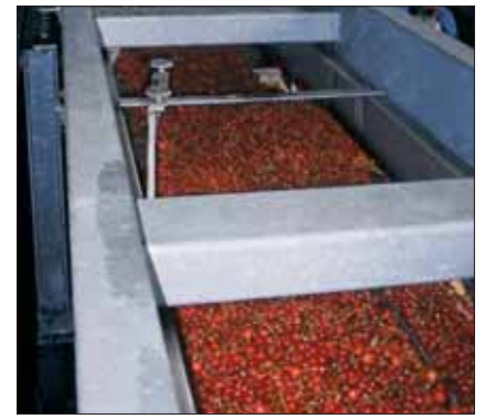
Fig. 32 Conveyor for handling raw cherries in a cannery
