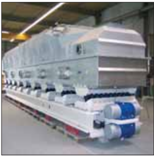
Fig. 7 The principle of the natural frequency system is also used to drive vibrating fluid-bed dryers
