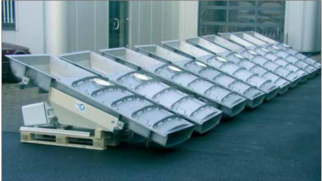
Fig. 7 Electromagnetic bin discharging troughs for transporting steamed rice between the steaming bins and the natural-frequency trough conveyors
