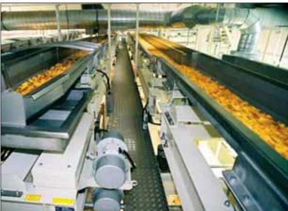
Fig. 3 Partial view of a vibrating conveyor plant with an overall length of 120 m used to convey potato chips at a rate of 60 m<sup>3</sup>/h
