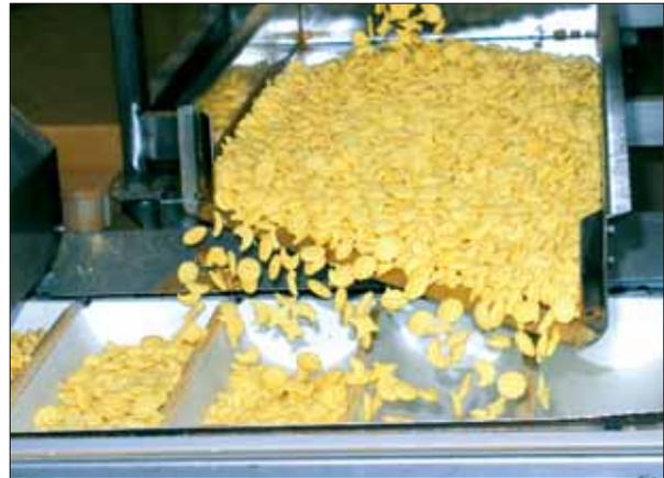
Fig. 2 Feeding to a vertical conveyor
