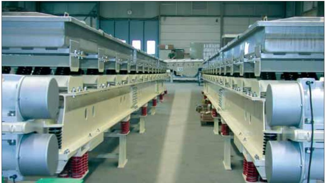
Fig. 8 Natural-frequency trough conveyors with a length of 20 m used to convey steamed rice at a rate of 40 t/h
