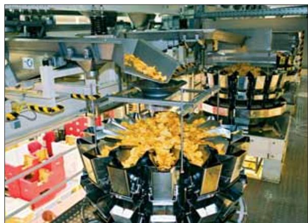
Fig. 6 Feeding the multiple-head balances and the packaging machines
