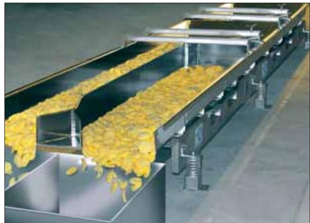
Fig. 4 Section of a conveying plant with electromagnetically activated vibrating trough conveyors
