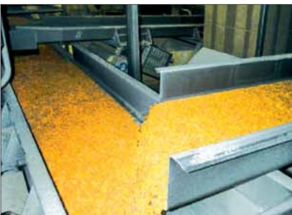
Fig. 5 Partial view of a vibrating conveyor plant with a length of 100 m used to convey cornflakes at a rate of 100 m<sup>3</sup>/h
