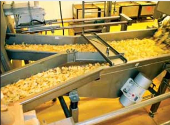
Fig. 1 Distributing trough for potato chips between the deep fat fryer and the flavor drums
