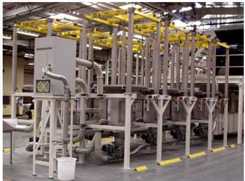
Complete emptying system: - dehumidifier - pneumatic conveying - hoist stretching system
