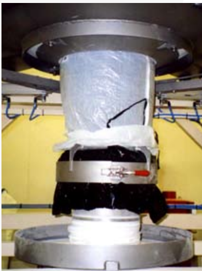
Inflatable seal ensures dust-free operation
