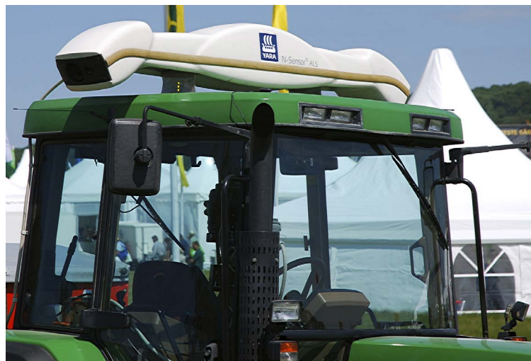
The Yara N-Sensor ALS mounted on this tractor's canopy records light reflection of crops, calculates fertilization recommendations, and then varies the amount of fertilizer spread. Photo by bdk, Wikimedia Commons/CC-BY-SA-3.0.
