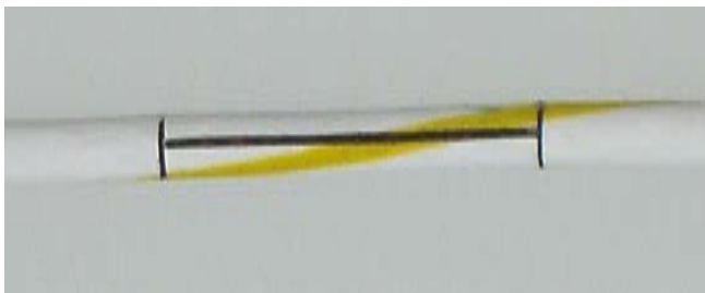
Above: 12 AWG, single core Polyimide and PTFE tape wrapped MIL spec aerospace wire (22759/87) with window strip and slit, with insulation left on.
