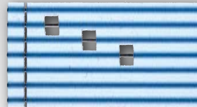
Flat ribbon cable, 18 mm (0.71") wide processed by a dual axis SIENNA system in a programmed pattern
