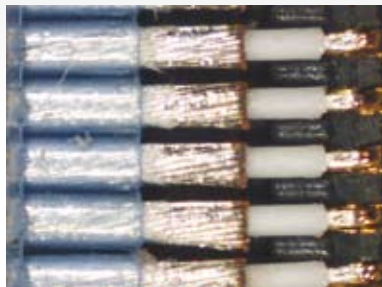
Left: Close-up of a laser scribed 42 AWG micro-coax ribbon cable used in mobile phone applications
