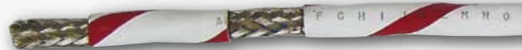
High temperature, shielded, twisted, 3-core cable, approx. 5 mm OD (0.2") used in aero engine harnesses with an end-strip and window strip performed on a SIENNA 530
