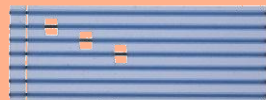
Flat ribbon cable, 18 mm (0.71") wide, end stripped by a dual axis SIENNA system
