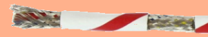
5mm OD high temperature shielded 3 core cable; end strip & window strip performed by a SIENNA 210D
