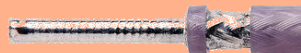
3mm (0.1") OD coaxial cable, end stripped and window stripped using a SIENNA 210D
