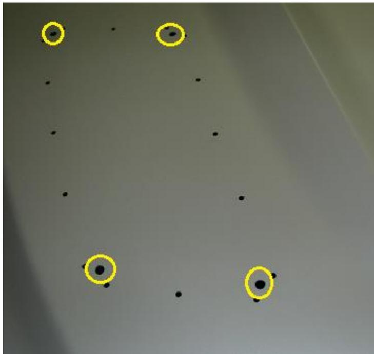
15) Clean each of these holes up from burrs with the countersink tool.
