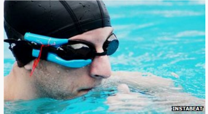
Instabeat is a heart rate monitor that can be attached to swimming goggles
