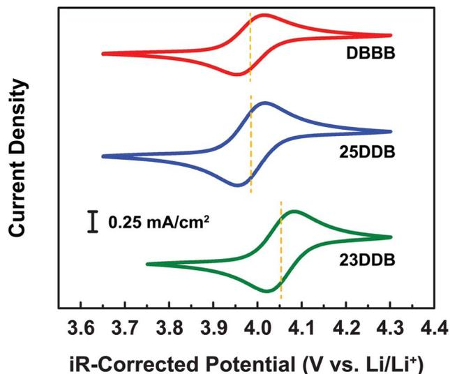
Fig. 2 Cyclic voltammograms of 2,5-di-*tert*-butyl-1,4-bis(2-methoxyethoxy)benzene (DBBB), 2,5-dimethyl-1,4-dimethoxybenzene (25DDB), 2,3-dimethyl-1,4-dimethoxybenzene (23DDB). All electrolytes consisted of 10 mM active species in 0.5 M LiTFSI/PC. The working, reference, and counter electrodes are glassy carbon electrode, fritted lithium metal, and unfritted lithium metal, respectively. The scan rate is 0.02 V s<sup>-1</sup>.
