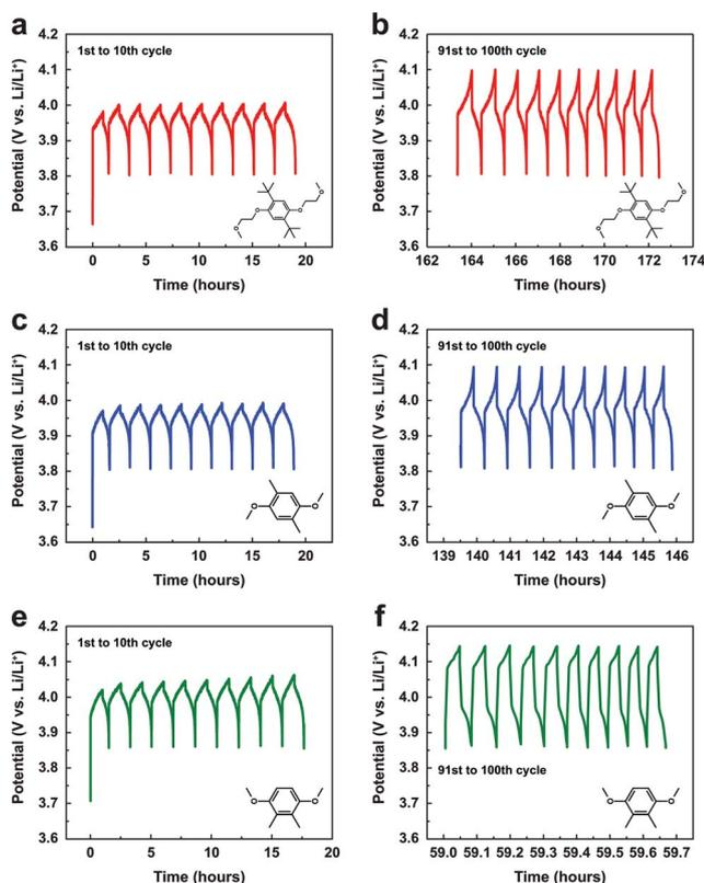
Fig. 4 Cycling profiles of DBBB (red), 25DDB (blue), and 23DDB (green) at 0.5 C from 0–50% state of charge for 1<sup>st</sup> to 10<sup>th</sup> cycle (a, c, e) and 91<sup>st</sup> to 100<sup>th</sup> cycle (b, d, f) in a bulk electrolysis cell. All electrolytes consisted of 1 mM active species in 0.5 M LiTFSI/PC and a total solution volume of 30 mL.
