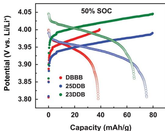
Fig. 3 Representative charge (solid circle)/discharge (open circle) cycles of DBBB (red), 25DDB (blue), and 23DDB (green) at 0.5 C from 0 to 50% state of charge in a bulk electrolysis cell. All electrolytes consisted of 1 mM active species in 0.5 M LiTFSI/PC and a total solution volume of 30 mL.
