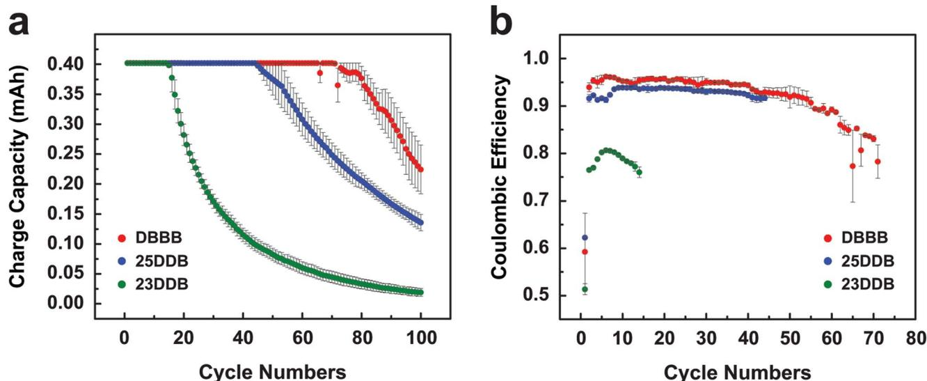
Fig. 5 (a) Charge capacity profiles for DBBB (red), 25DDB (blue), and 23DDB (green) with respect to the cycle number based on the data from Fig. 4. (b) Coulombic efficiencies of the plateaued region on the corresponding capacity profile. Data shown represents the average of two independent experiments for each compound.
