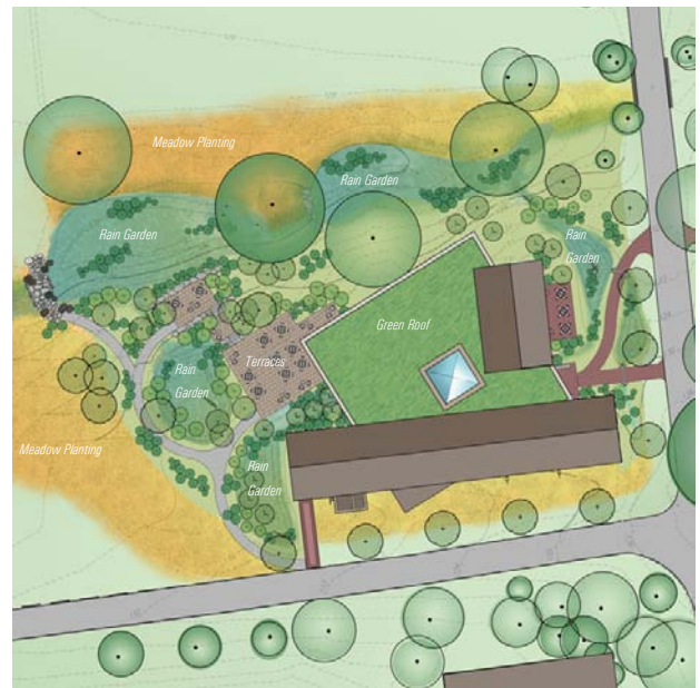
Three western terraces, a small eastern terrace and entrance walk are set into a woodland garden overlooking a series of rain gardens. The large library reading room has a green roof.
