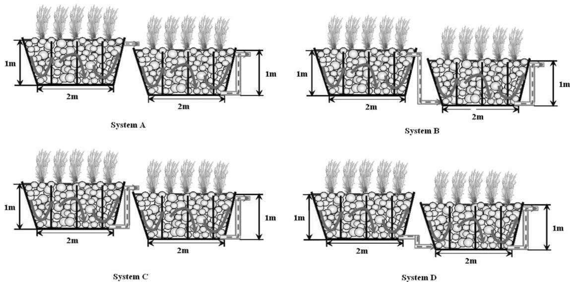
**Fig. 3** Different types of constructed wetlands for hydroponic waste solution treatment. *System A* Up-Up stream; *System B* Up-Down stream; *System C* Down-Up stream; *System D* Down-Down stream (Park et al. 2012)
