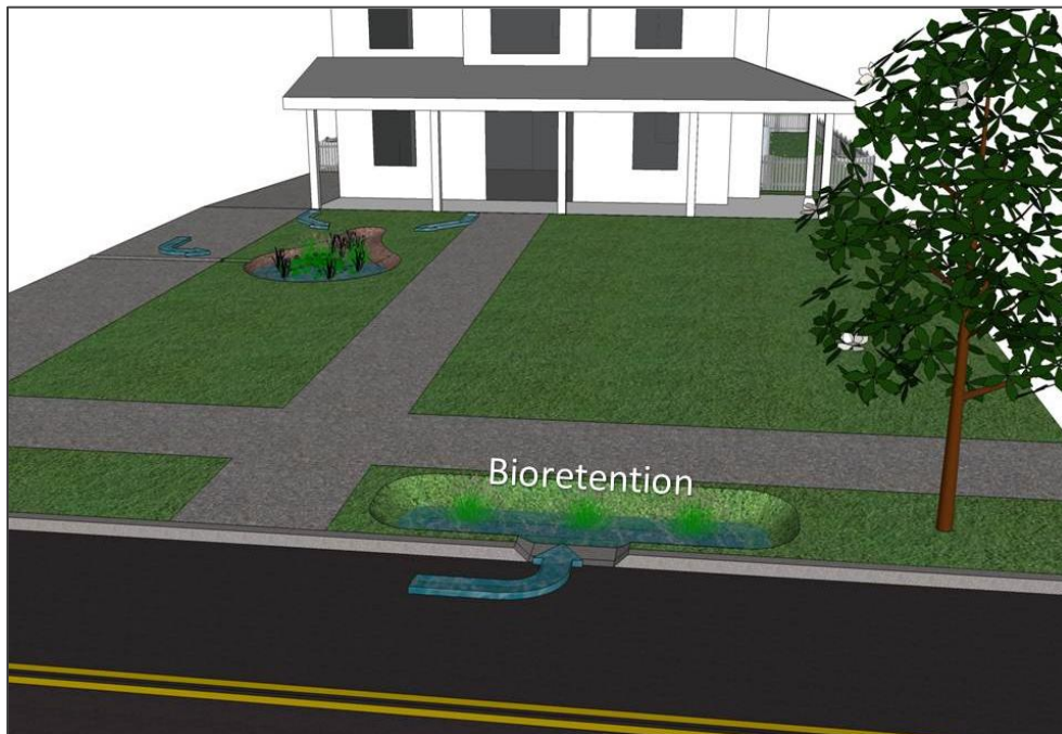
Figure 17: Street-side bioretention capturing runoff from the yard, sidewalk, driveway, and street
