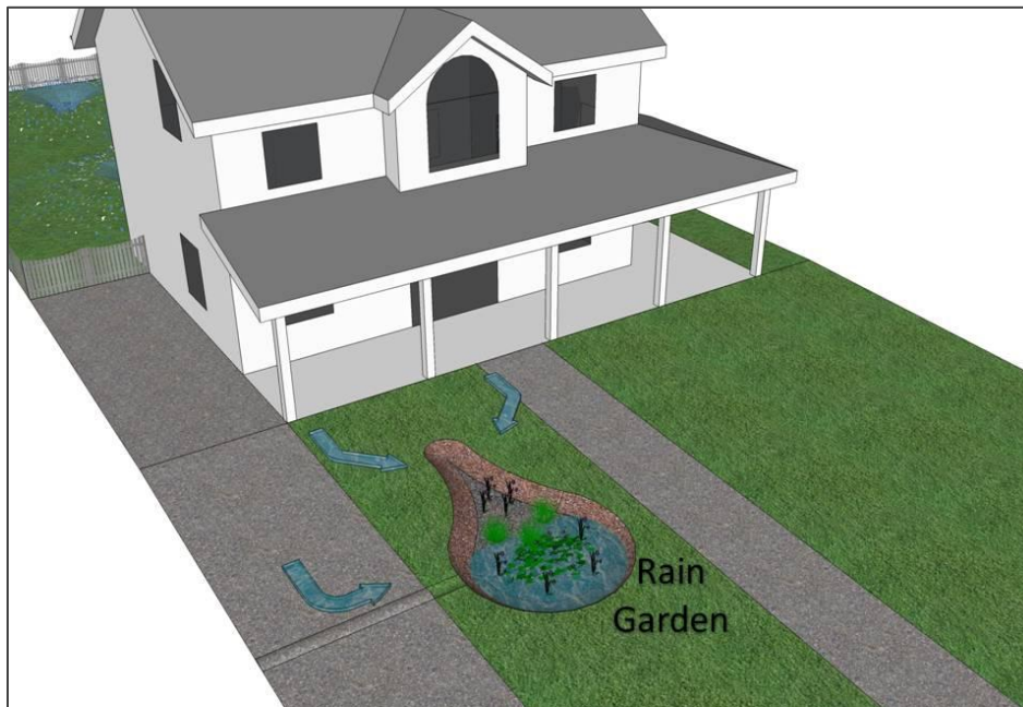
Figure 16: Rain garden constructed on a front yard capturing runoff from the rooftop, driveway, and sidewalk
