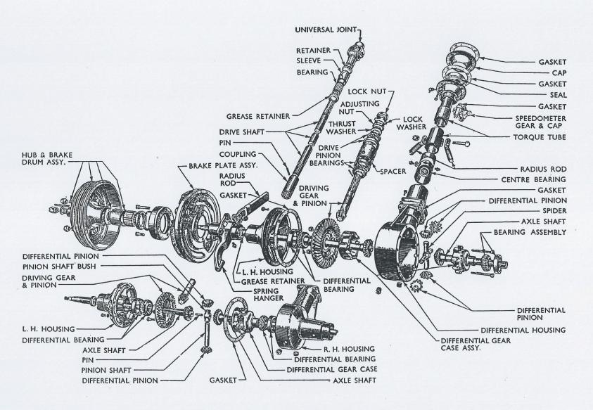
The differential assembly on the right-hand side of the illustration applies to the 10-cwt van.
