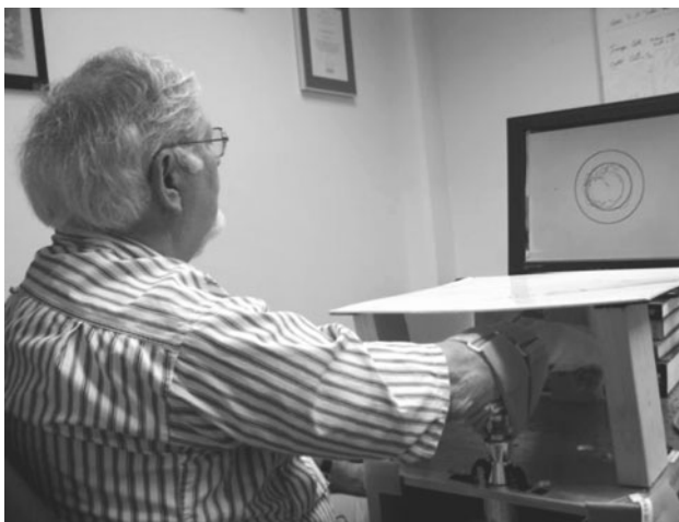
Fig. 1 The experimental setup. The participant performs 1-dimensional horizontal flexion/extension movements with the forearm to control a cursor displayed on a phase plane, where velocity is plotted versus position
