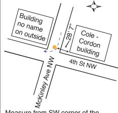
Measure from SW corner of the Cole - Cordon building 28' 7" west inline with sawcut joint in concrete out into McKinley Ave NW
