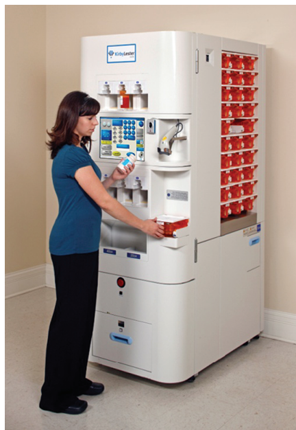
Figure 3-4. Robotic dispensing machine fills and labels prescriptions. Photo courtesy of Kirby Lester, LLC.
