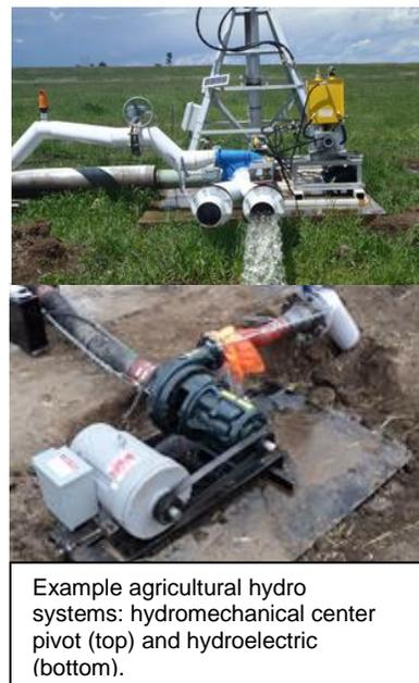
Example agricultural hydro systems: hydromechanical center pivot (top) and hydroelectric (bottom).
