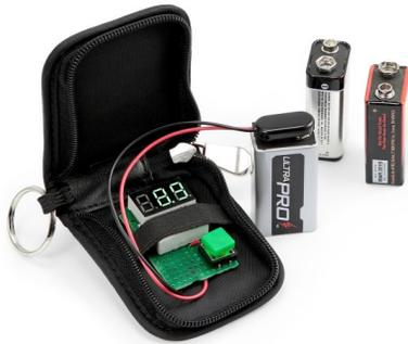
The E-Lock Battery Analyzer is designed to test 9-volt batteries *under load* by simulating the power demands of an electronic safe lock during an open/close cycle. It will tell you immediately if a particular battery will perform properly in modern motorized or solenoid-based electronic locks.
