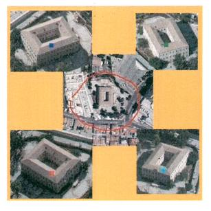
The system, called Oblivision, is from <u>Idan Computers Ltd.</u>, based in Israel. The solution combines ordinary orthophotos and digital terrain models with oblique images. Once a spot is selected (by clicking on the orthophoto, supplying coordinates, an address etc), the system provides views of the spot from all directions. Analysis and measuring can be done on the individual oblique photos. Heights of poles can be measured, or the length of a guard rail, for example.
