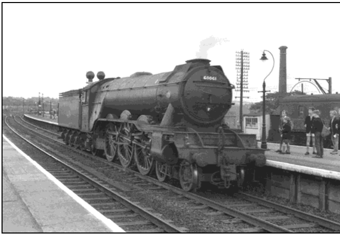
Two views of Kings Cross A3 60061 Pretty Polly : on 28/7/1961, the A3 wore 'trough' type smoke deflectors around her chimney.
